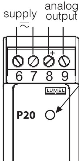
Diode of the transducer work state:
