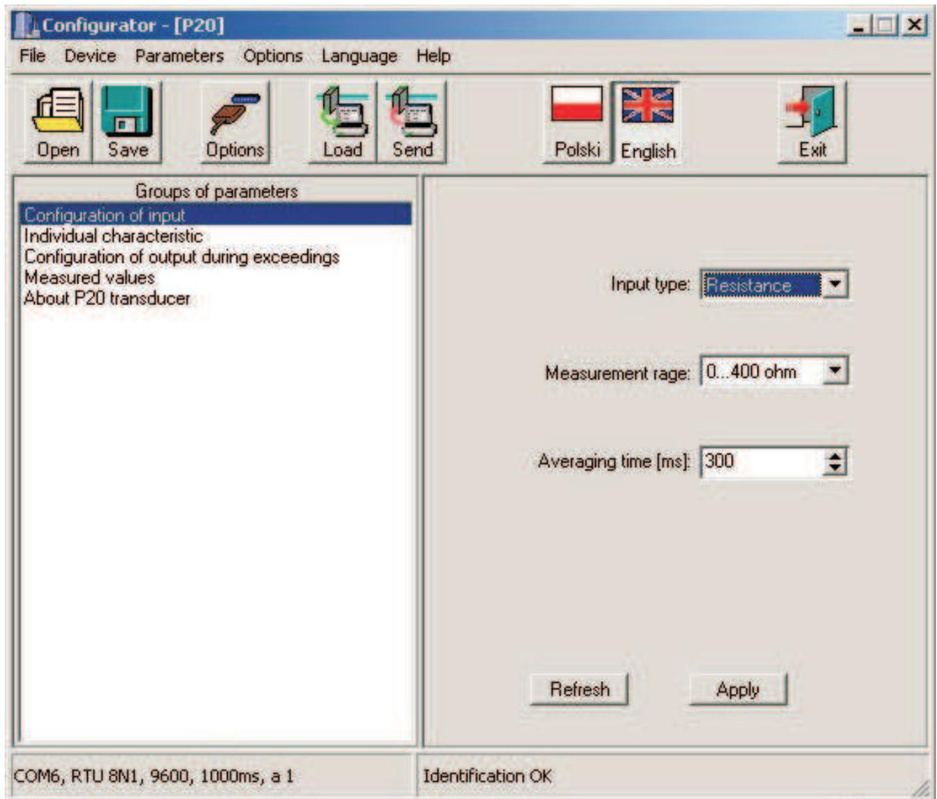
Fig. 4. View of the LPCon program window “Input configuration”
