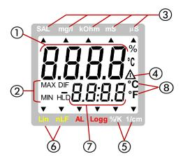
Main display: conductivity, resistivity, filtrate dry residue (TDS), salinity or user prompt
