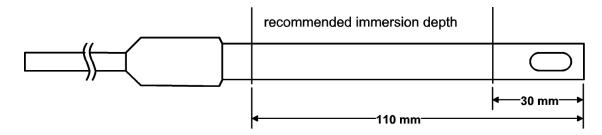
The measuring cell can either be stored dry or in water. After dry storage wetting time will be prolonged slightly. If changing over from one liquid to another with conductivities varying widely make sure to properly rinse and shake dry measuring cell.
